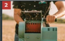
2 Built-in threshing drum and interchangeable concaves for use in multiple cereal and oil seed crops.
