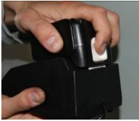
Figure 1: Installing battery in charger
