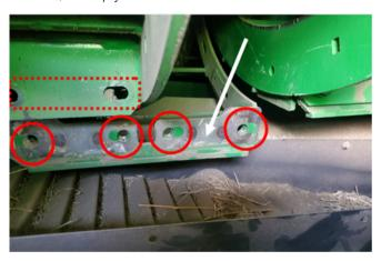
Step 2 - Remove the 1st and 2nd position OEM concaves.
