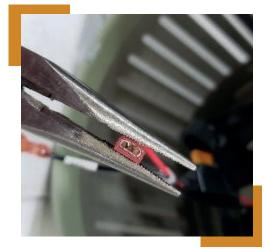
Note: Before attaching the spade connectors, use pliers to compress the female harness terminals. This will allow them to make a tight connection.
